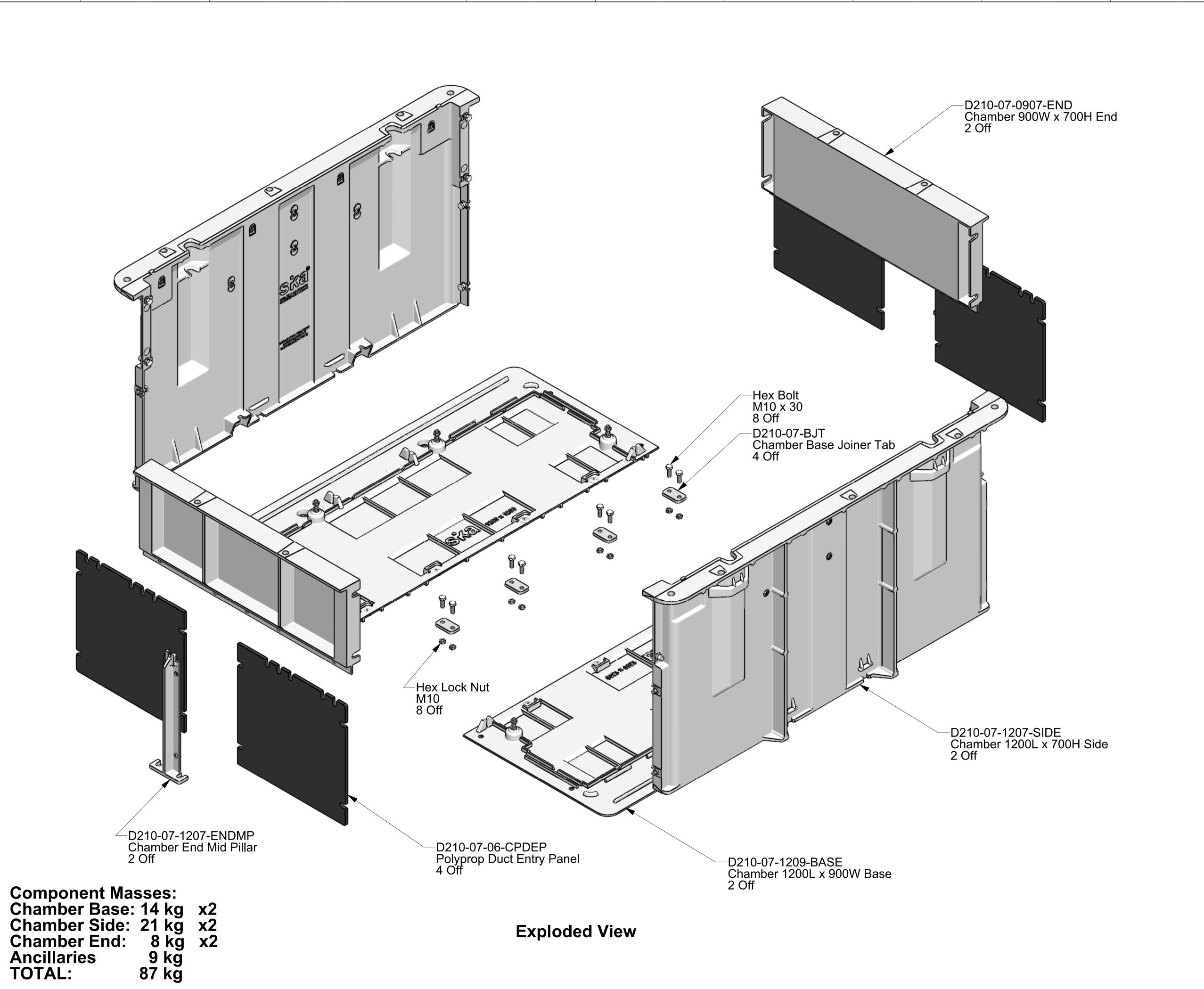
CLIENT PROJECT: Aluminium Jointing Chamber To Class D210 kN Loads To AS 3996 : 2006 TITLE: Chamber 1200 x 900 x
