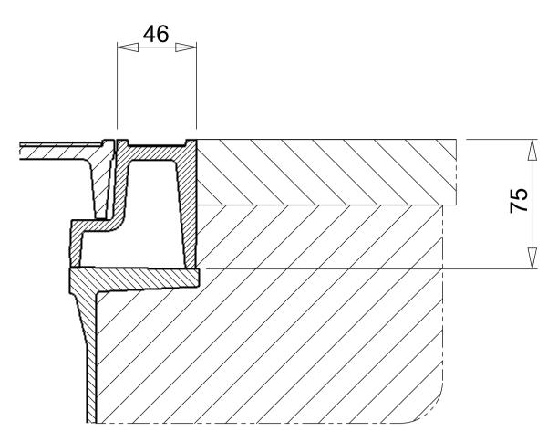
Typical Installation Frame Supported By Chamber / Extension Flange
